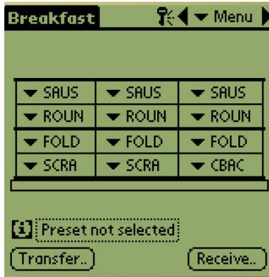
**Step 15:** Beam over the cabinet configurations with a Palm, which holds the restaurant's desired cabinet configurations by opening the UHC-P software to the setup window.
