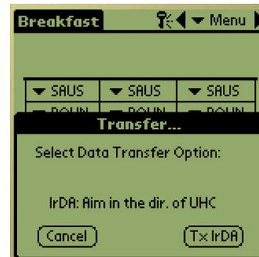
**Step 16:** Ensure the dark receiving lens on the front of the UHC-P cabinet is clean. Hold the Palm Pilot parallel with the floor and aim it at the lens from no more than one foot away.
