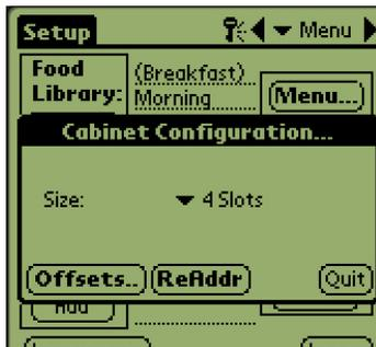
**Step 5:** The Cabinet Configuration screen is displayed. Make sure that the proper slot size is displayed: (2 slots, 4 slots, narrow). (**NOTE:** The button-push sequence for the Narrow unit is different and covered in Steps 7N-14N on the adjoining page.) With the Palm horizontal and near the lens on the UHC-P cabinet, tap the ReAddr button in the bottom center of the screen.
