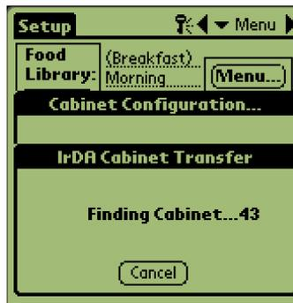
**Step 6:** The addresses of the cabinet's boards will be beamed to the cabinet. A success message will display when the process is complete. **Press 1 Button** will be displayed on each slot.
